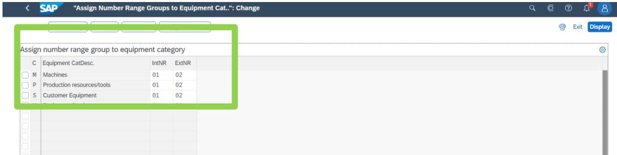
Now existing assignment of the NR keys can be adjusted. Here in the case equipment category P is assigned with a different key than initially assigned. Once changes done click on save button at bottom right corner.
